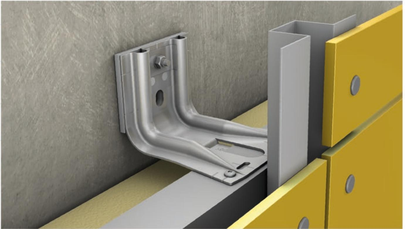
Over 40 years ago, the SPIDI® facade system was designed for secure, quick, and easy facade installation. Since then, the system has been expanded, adapted to growing insulation thicknesses, and steadily improved.
