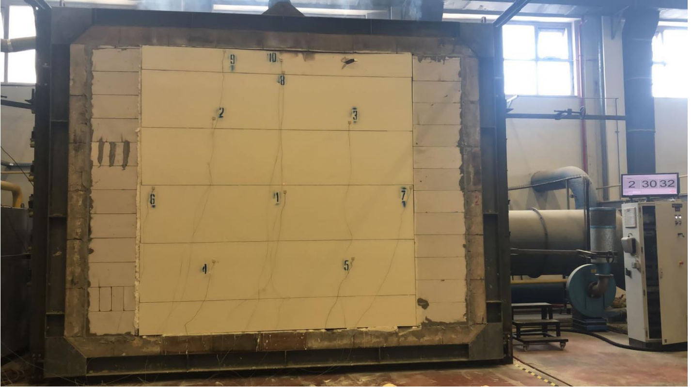
Figure 9 – At the end of the test Unexposed Side
