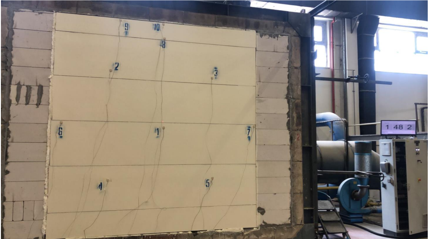
Figure 8– During the Test Unexposed Side
