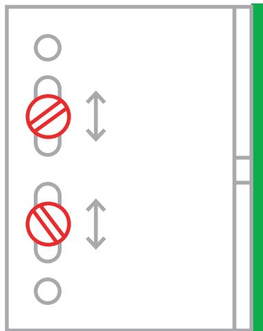
**Please note:** Please note: the correct fixed and sliding points on the helping hand bracket must be used. After adjustments are made for line and level, they are fixed using self-drilling stainless steel screws, SR2 (4.2 X16).
