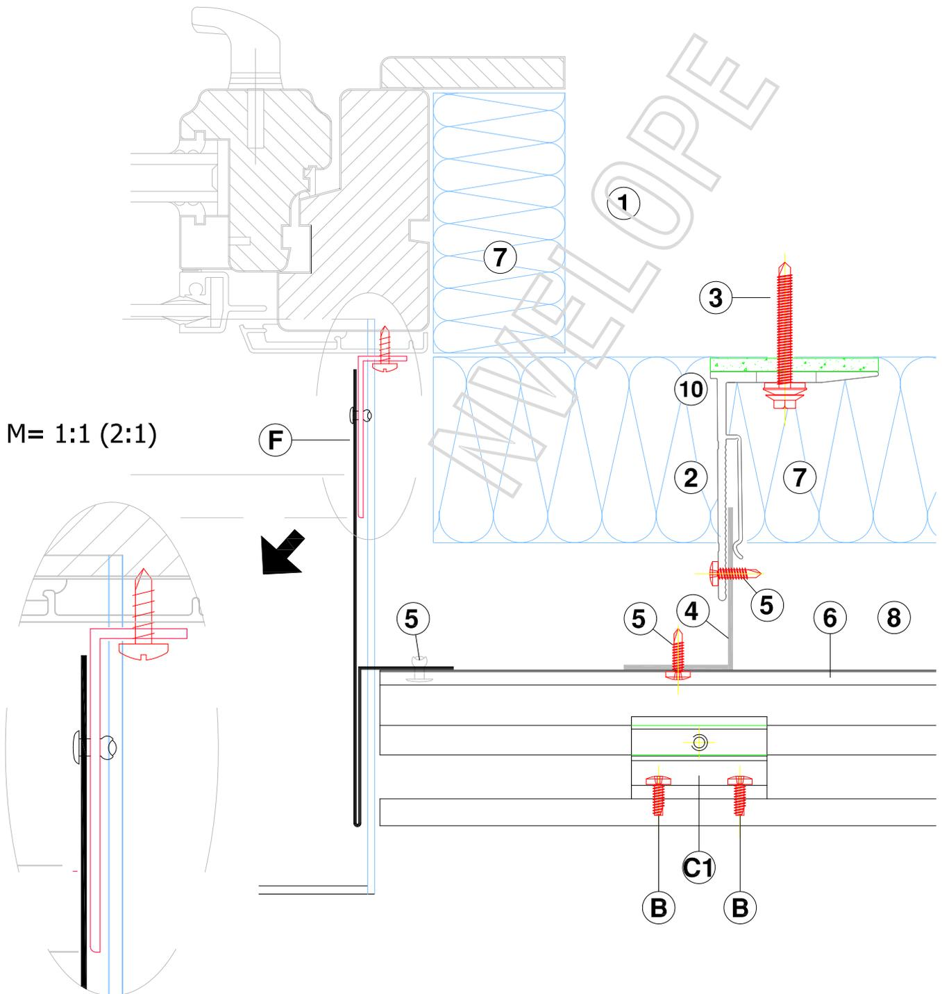
HORIZONTAL SECTION - WINDOW JAMB DETAIL
