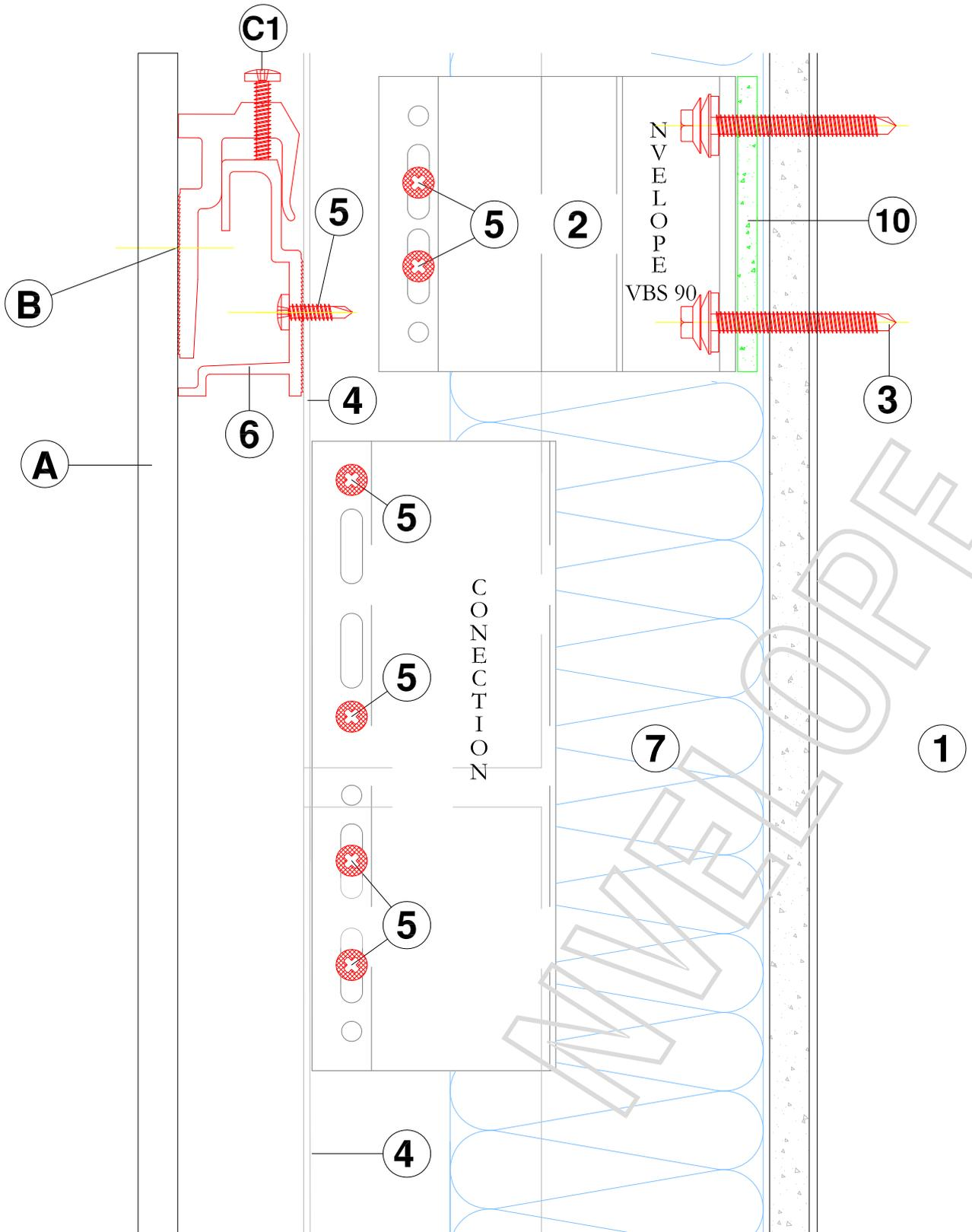
VERTICAL SECTION - CONNECTION PIECE - JOINING OF PROFILES
